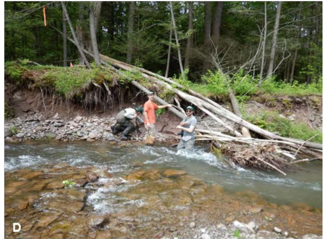
Figure 8. Documentation of WC2 site at WC-BEMS-02 on Warner Creek. Photo A depicts mass failure of glacial lake sediment and terrace alluvium. Photo B depicts where the stream is eroding into glacial lake sediment. Photo C illustrates the mass wasting terrace with glacial lake sediment exposed in the channel margin. Photo D illustrates headcut into glacial lake sediment in streambed.
